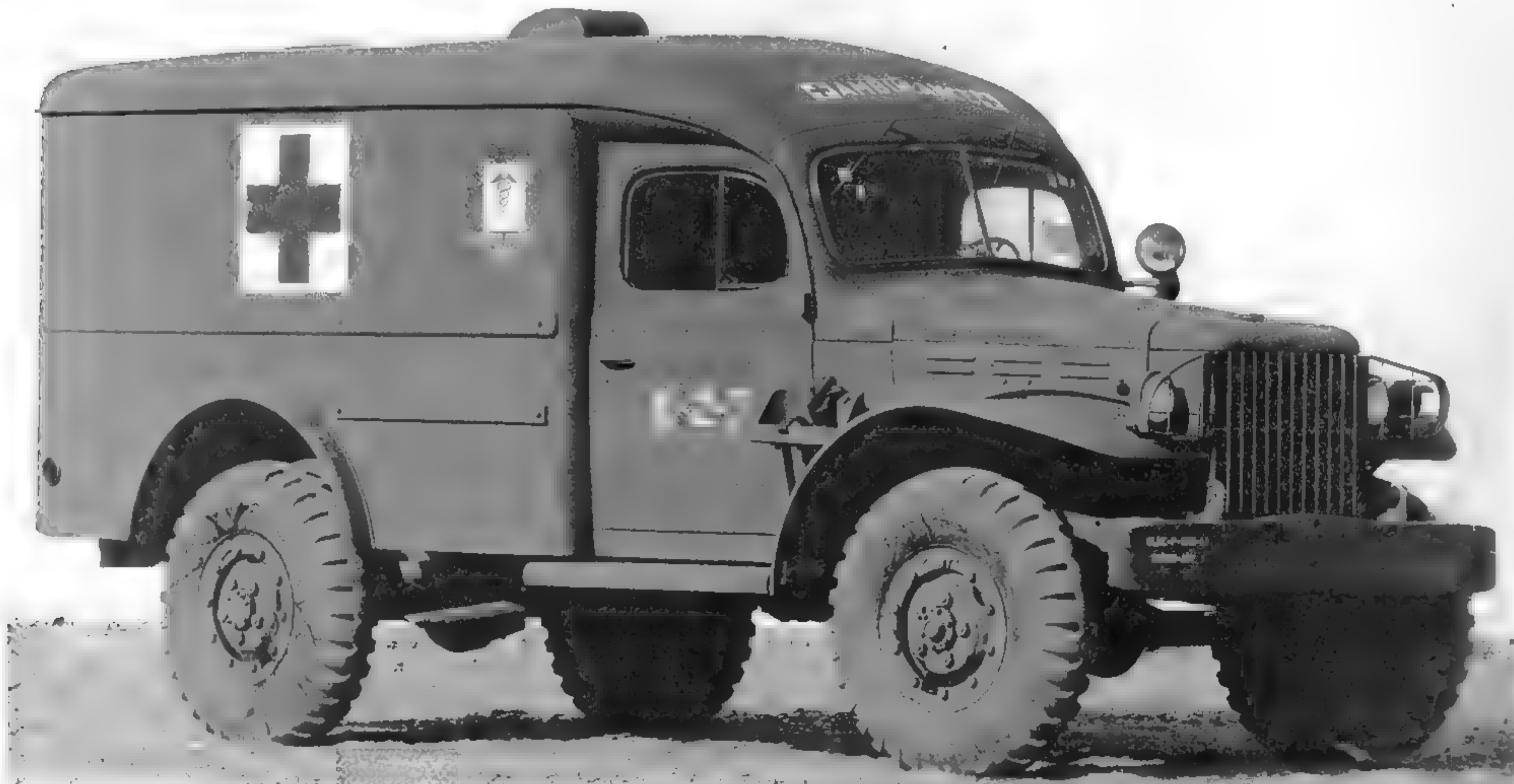
The WC-54 was the initial ambulance built on the G-502 chassis, and it became familiar to many wounded GIs. Notice the vent glass in the door, which is not present in the similar door fitted to the carryall. Often the two doors types were interchanged, but the vented window is only truly correct on the ambulance. (U.S. Army photo)
